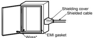
\* These wires are used to improve the conductivity between the door and control cabinet.
