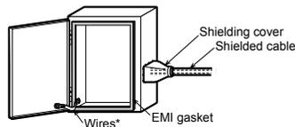
\* These wires are used to improve the conductivity between the door and control cabinet.
